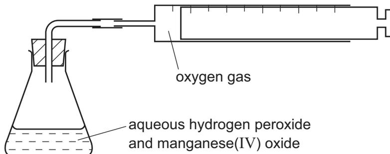
40 cm<sup>3</sup> of aqueous hydrogen peroxide was put in the flask and 0.1 g of small lumps of manganese(IV) oxide was added. The volume of oxygen collected was measured every 30 seconds. The results were plotted to give the graph shown below.
